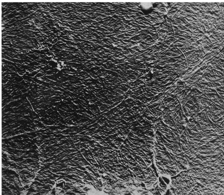
Fig. 10. An electron micrograph of sisal after extracting lignin from the wall. Magnification = 20000 \times .
