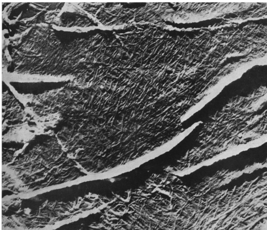
Fig. 2. An electron micrograph of the primary wall of a ramie fiber. Adhering non-cellulosic substances give to the fibers of this and certain other photographs a somewhat diffuse appearance. Magnification = 20000 \times .
