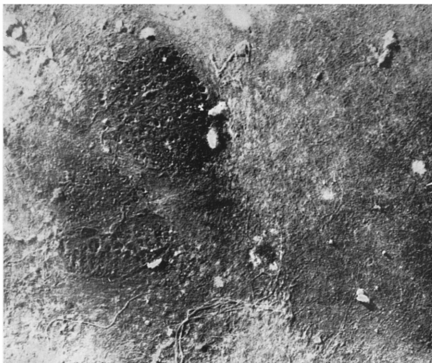
Fig. 9. An electron micrograph of sisal. A layer deposited deeper in the wall. Magnification = 20,000
