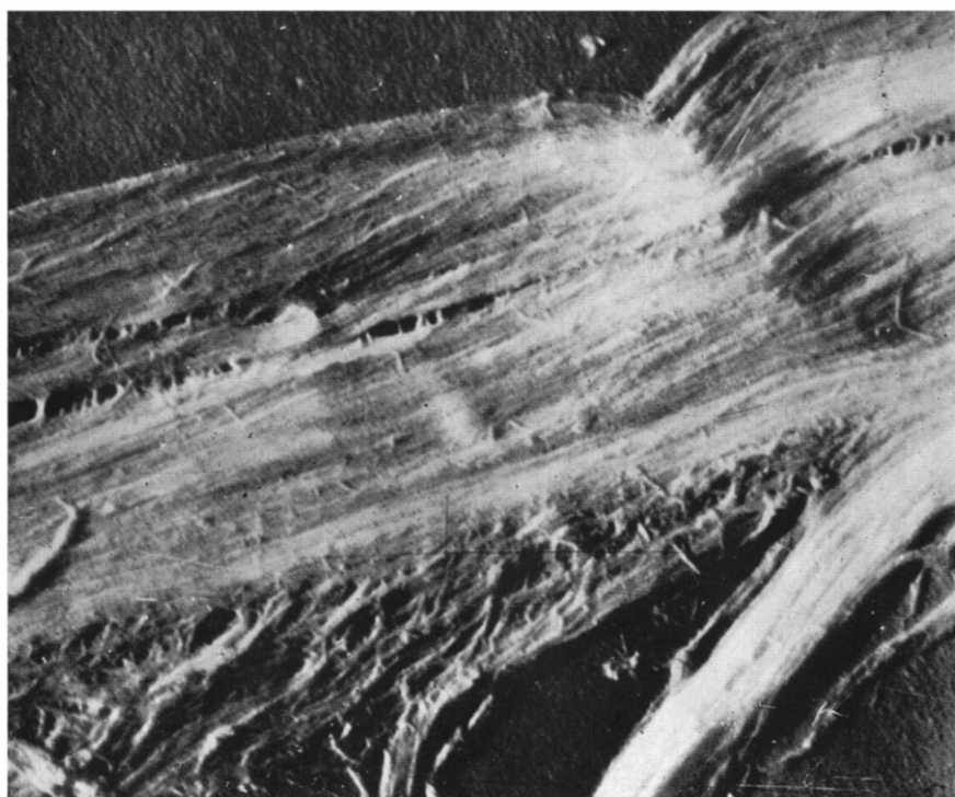
Fig. 5. An electron micrograph of the secondary wall of a cotton fiber. Magnification = 20000 X
