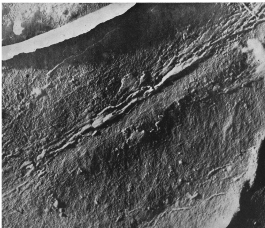
Fig. 8. An electron micrograph of sisal. The interior wall is heavily impregnated with lignin Magnification = 20000 \times .
